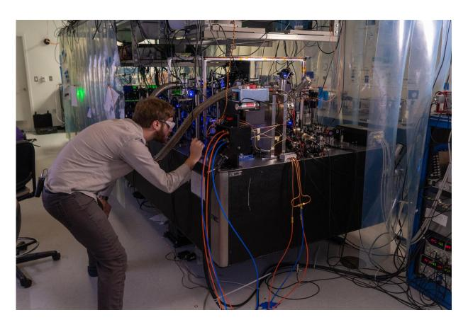
Rice University graduate student Tom Langin works at the laser table where beams of various wavelengths were used to make the world's first laser-cooled neutral plasma. (Photo by Brandon Martin/Rice University) Credit: Brandon Martin/Rice University
