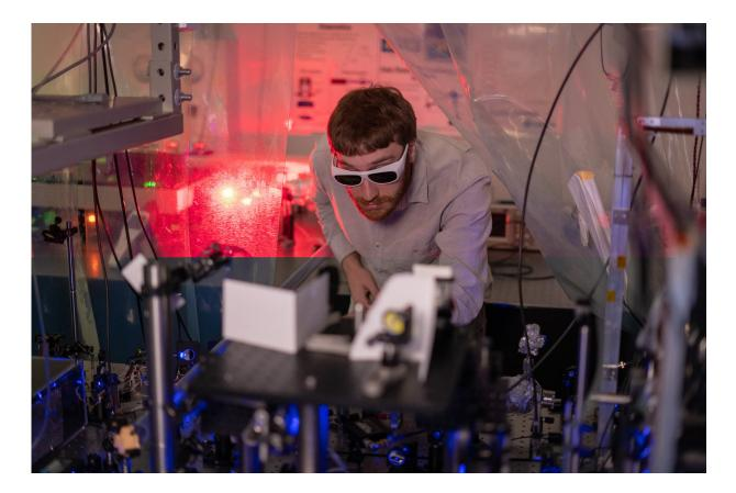
Rice University graduate student Tom Langin makes an adjustment to an experiment that uses 10 lasers of varying wavelengths to laser-cool ions in a neutral plasma. (Photo by Brandon Martin/Rice University) Credit: Brandon Martin/Rice University
