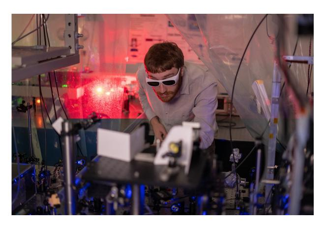
Rice University graduate student Tom Langin makes an adjustment to an experiment that uses 10 lasers of varying wavelengths to laser-cool ions in a neutral plasma. (Photo by Brandon Martin/Rice University) Credit: Brandon Martin/Rice University
