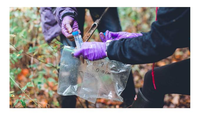
Graduate students in Peter Jaffe's research group take soil samples from along the Neuse River and its tributaries. Back at their lab in Princeton, the researchers examine the samples to understand a chemical process called Feammox, a potential breakthrough in eliminating nitrogen pollutants. Credit: Christobal Perez/Azul Photography
