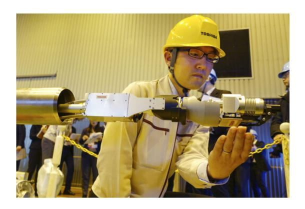
Toshiba Corp.'s energy systems unit group manager Jun Suzuki shows a remote-controlled melted fuel probe device at its facility in Yokohama, near Tokyo, Monday, Jan. 28, 2019. Toshiba unveiled the device carrying tongs that comes out of a long telescopic pipe for an internal probe in one of three damaged reactor chambers at Japan's tsunami-hit Fukushima nuclear plant - this time to touch chunks of melted fuel. (AP Photo/Mari Yamaguchi)
