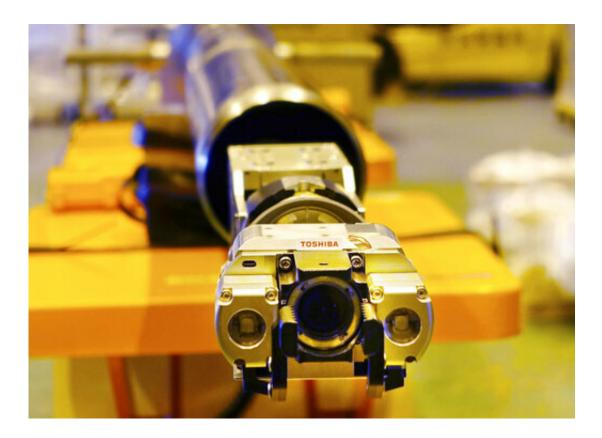
A remote-controlled melted fuel probe device is unveiled by Toshiba Corp. at its facility in Yokohama, near Tokyo, Monday, Jan. 28, 2019. Toshiba unveiled the device carrying tongs that comes out of a long telescopic pipe for an internal probe in one of three damaged reactor chambers at Japan's tsunami-hit Fukushima nuclear plant - this time to touch chunks of melted fuel. (AP Photo/Mari Yamaguchi)
