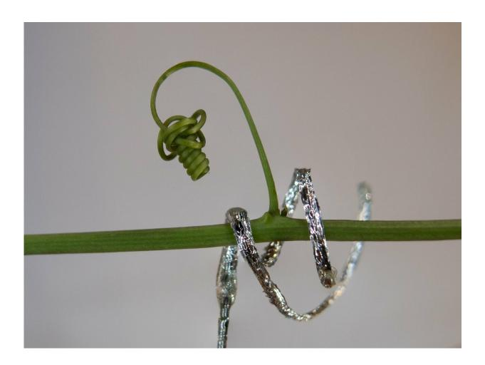
The tendril-like soft robot is able to curl around Passiflora caerulea plant stalk. It is able to curl and climb, using the same physical principles determining water transport in plants. Credit: IIT-Istituto Italiano di Tecnologia
