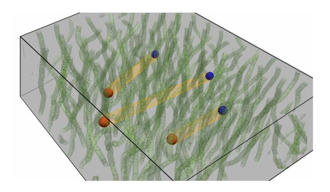
A 3D superinsulator, in which vortex condensate (green lines) squeezes the electric field lines connecting charge-anticharge pairs (red and blue balls) into the electric strings (orange strips). These strings tightly bind these charge-anticharge pairs, completely immobilizing them, so electric current cannot be produced. Credit: Argonne National Laboratory
