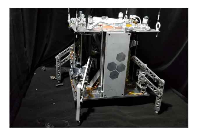
By using steam rather than fuel, the World Is Not Enough (WINE) spacecraft prototype can theoretically explore "forever," as long as water and sufficiently low gravity is present. Credit: University of Central Florida
