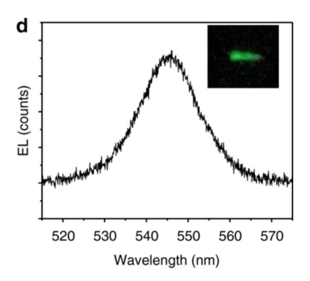
The wavelengths of light emitted from the spintronic LED. The inset shows the green light from the device. Credit: University of Utah
