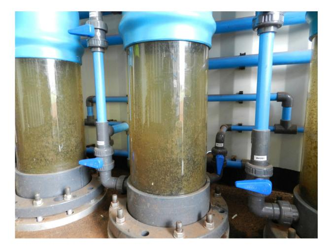
Coagulation and flocculation columns for purifying the river water. Credit: Fraunhofer-Gesellschaft
