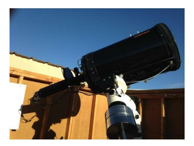
IoIO consists of a 14-inch (35 cm) Celestron Schmidt-Cassegrain telescope feeding a custom-built coronagraph. An Astro-Physics 1100 mount, 80mm offset guide scope, and associated software enable the system to acquire and guide on Solar System targets robotically. Credit: Planetary Science Institute
