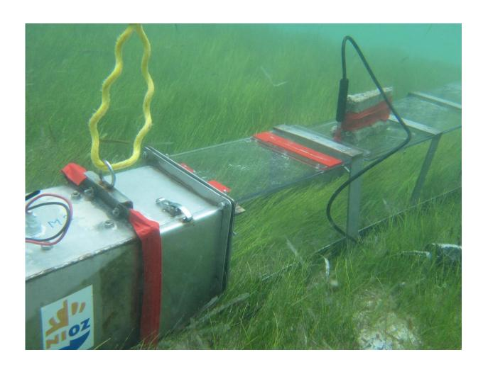
A portable water flume designed at NIOZ was used to measure the ability of seagrass to keep sand in place and prevent erosion. Credit: Rebecca James
