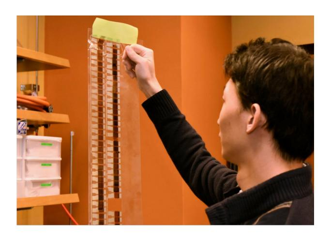
Dr. Longbin Qiu holds up a sheet of solar cells made from flexible materials. The Energy Materials and Surface Sciences Unit aims to develop these devices to craft solar curtains and solar technologies that can be easily incorporated into people's homes. Credit: Okinawa Institute of Science and Technology
