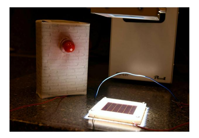
The Energy Materials and Surface Sciences Unit has fabricated new Perovskite Solar Cell modules with optimized stability and efficiency. A prototype is shown here powering a small fan. Credit: Okinawa Institute of Science and Technology
