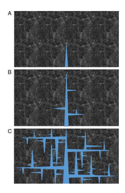
Schematic branching due to natural fractures. (A) Water is injected at high pressure through damaged zones and weak layers, (B) crack branch-ing initiates due to the presence of damaged zones and natural fractures, and (C) dense
