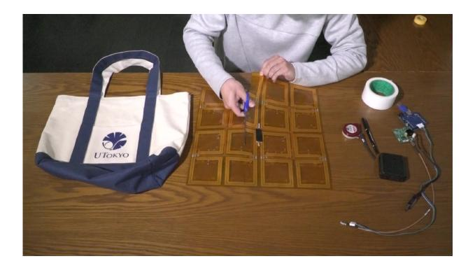
As the charger can be reshaped it could be incorporated into various portable objects Credit: Kawahara Laboratory
