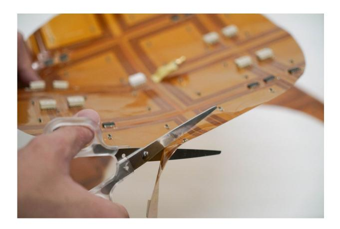
The charger still functions after it's cut due to a wiring method known as H-tree wiring Credit: (c)2018 Kawahara Laboratory
