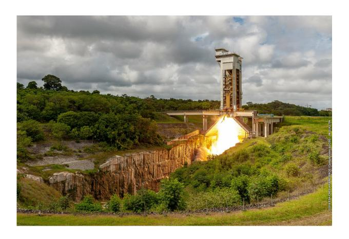
On 28 January 2019, the first qualification model of the P120C solid-propellant motor, in the configuration for Vega-C, was static fired on the test stand at Europe's Spaceport in French Guiana. During a burn time of 135 seconds, the P120C delivered a maximum thrust of 4650 kN. No anomalies were seen and the performance met expectations. Credit: ESA/CNES
