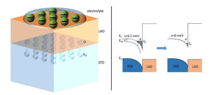
(Left) Schematic illustration of the operation of LAO/STO electrolyte field effect device. The presence of high electric field drives the oxygen atoms (O) migration into the STO layer to fill some of the vacancies (VO). (Right) Schematic band diagrams of the LAO/STO interfaces showing the change in interfacial energy band structures as a result of electrolyte field effect. Credit: Physical Review Letters
