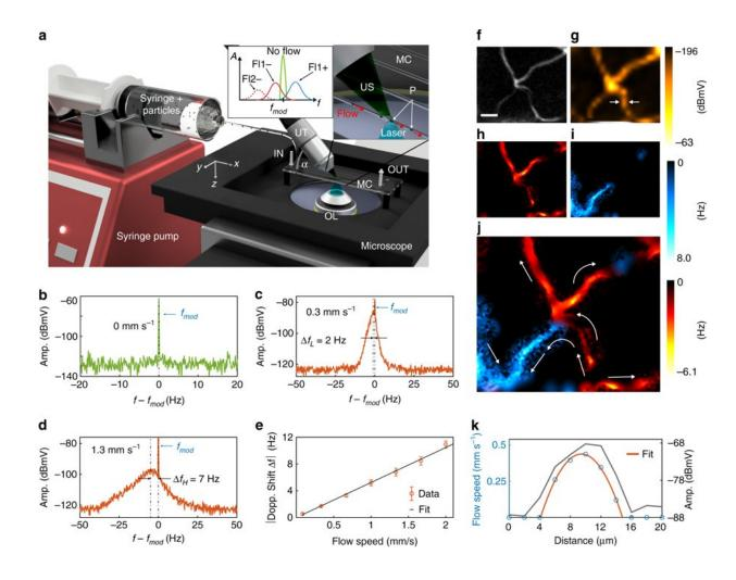
Optoacoustic imaging of microcirculatory blood flow in a mouse ear in vivo. a A scheme of the  $\mu$ Doppler detection set-up. FL1– flow 1 away from the US sensor, FL2– flow 2 away from the US sensor (FL2–
