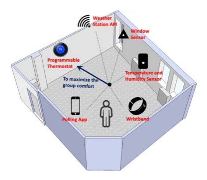
A multi-sensor system monitors the environment and room occupants, and adjusts the room heat and cooling accordingly. Credit: Carol Menassa, et al., <a href="CC">CC</a>
