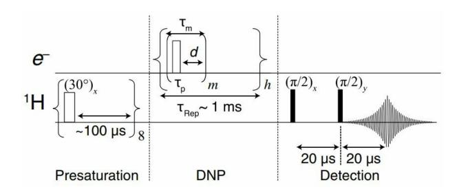
Schematic diagram of a TOP-DNP sequence performed at 0.35 T. The TOP-DNP pulse sequence is composed of a train of m microwave pulses of a length  $t_p$  separated by a delay d in between the pulses, in static (nonspinning) samples. The sequence is repeated h times with a repetition time  $t_{Rep}$  to build up bulk  $^1H$  polarization. The sequence becomes pulsed SE if d = 0. Credit: *Science Advances*, Tan et al., *Sci. Adv.* 2019;5: eaav6909
