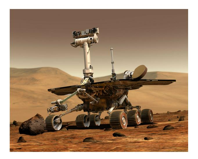
This illustration made available by NASA shows the rover Opportunity on the surface of Mars. The exploratory vehicle landed on Jan. 24, 2004, and logged more than 28 miles (45 kilometers) before falling silent during a global dust storm June 2018. There was so much dust in the Martian atmosphere that sunlight could not reach Opportunity's solar panels for power generation. Credit:
