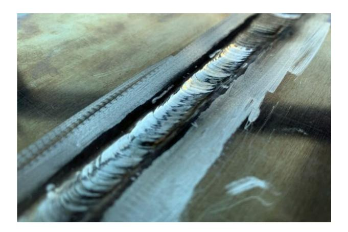
Two pieces of aluminum alloy 7075 welded together using a nanoparticleenhanced filler wire. Credit: Oszie Tarula/UCLA
