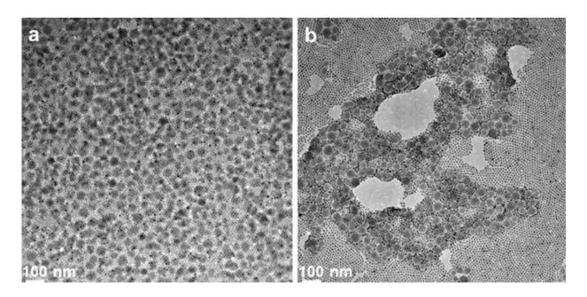
TEM images of MOFs and iron-oxide nanocrystals self-assembling into a bilayer film. Credit: Jeff Urban et al./Berkeley Lab
