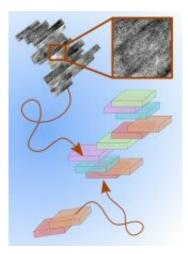
Scheme of transport and aggregation of boehmite nanoplatelets. Cryogenic transmission electron microscopy shows platelet stacks that align and merge into single crystals. Credit: Environmental Molecular Sciences Laboratory
