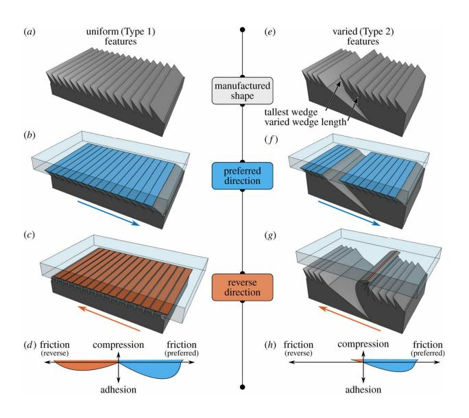
A comparison between uniform features (Type 1), left, and a group of features which exhibits one-way friction (Type 2), right, with resulting force-space plots showing performance, bottom. In the neutral state (a), the Type 1 features are all
