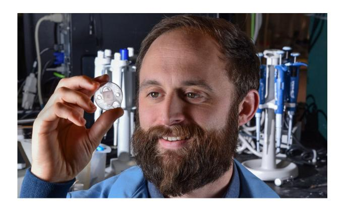
Sandia National Laboratories researcher Philip Miller examines a microneedle device. The new device design uses an array of needles and can extract 20 microliters of interstitial fluid, compared to the two microliters that the previous version of the device achieved. Credit: Randy Montoya
