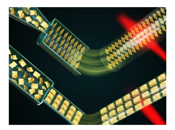
Sheet alignment and orientation order of graphene structures induced by microfluidics design enable the microstructure control and optimization of thermal-mechanical and electronic properties of macroscopic graphene fibers. Credit: Rensselaer Polytechnic Institute
