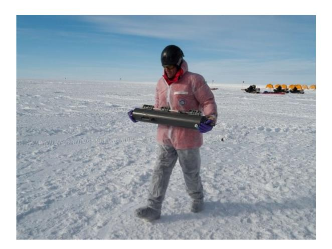
In this file photo, Montana University System Regents Professor John Priscu takes a Niskin bottle water sampler to a lab at an Antarctic field site for anaysis. Priscu, a polar scientist in MSU's College of Agriculture, is once again in the Antarctic, this time looking for living organisms in Mercer Subglacial Lake, located 4,000 feet below the Antarctic ice sheet. Credit: JT Thomas
