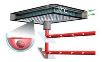
A multiwell plate where each well contains tumor tissue is placed on an inverted microscope held at 37°C. A laser beam is focused on one area of the tumor, then moved to achieve a mapping. The diffused light is collected by the microscope lens and analyzed in an interferometer to detect wavelength variations (in other words, "color" variations). Credit: Jérémie Margueritat/ILM/CNRS
