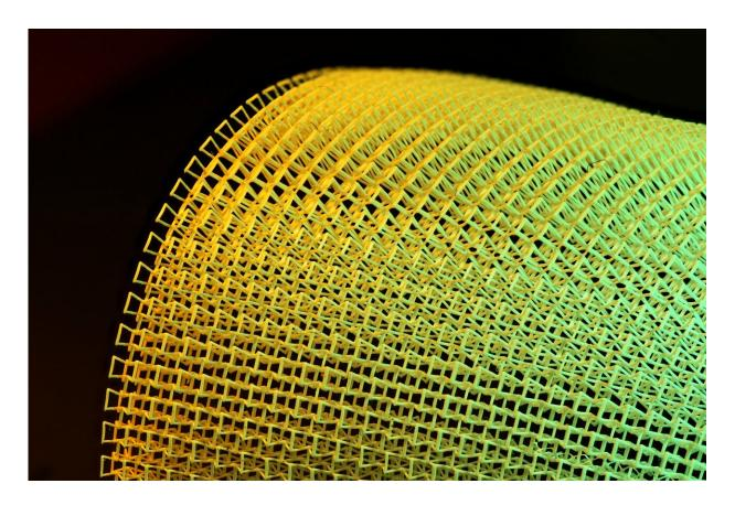
The printed flexible sheet of piezoelectric material. Credit: Virginia Tech
