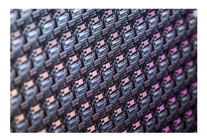
Fraunhofer IAF develops electronic components and systems based on GaN. The image shows a processed GaN wafer. Credit: Fraunhofer Institute for Applied Solid State Physics IAF
