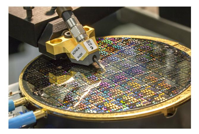
A team of researchers at Fraunhofer IAF has been working on the piezoelectric properties of ScAlN for the use in high-frequency filters for many years. The picture shows the characterization of such devices on a wafer. Credit: Fraunhofer Institute for Applied Solid State Physics IAF
