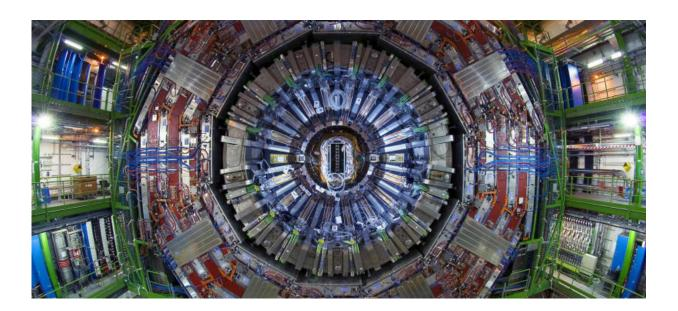
The Compact Muon Solenoid detector is a general-purpose detector at the Large Hadron Collider (LHC) in Switzerland, designed to observe any new physics phenomena that the LHC might reveal. Credit: CERN
