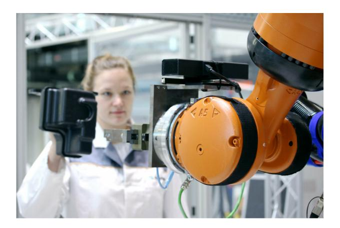
The robot detects the component in the worker's grasp and cautiously follows it until she hands it over. Credit: Fraunhofer IWU
