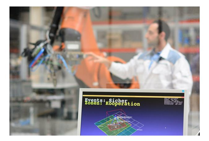
Various safety zones around the robot determine wether and how robot and human can work together in each zone. Credit: Fraunhofer IWU
