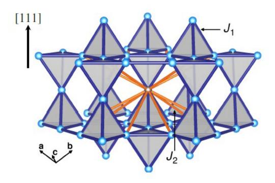
The model refers to a cubic crystal structure (pyrochlore lattice). Not only were magnetic interactions between the nearest neighbours included, but also with the next nearest neighbours (see drawing). Credit: HZB
