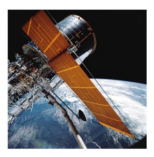
In this April 25, 1990 photograph provided by NASA, most of the giant Hubble Space Telescope can be seen as it is suspended in space by Discovery's Remote Manipulator System (RMS) following the deployment of part of its solar panels
