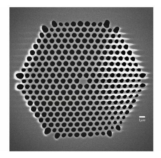
This image shows an electron-microscope picture of the interior of one of the researchers' fibres. The fibres are sophisticated photopic-crystal fibres. They are as thin as a human hair and inside they carry hole structures that guide the light in the centre. Credit: Drori et al.
