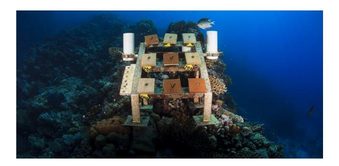
The researchers determined the overall accretion or erosion rate by deploying limestone blocks like these pictured at sites 3, 10, and 25 kilometers from the shore and by measuring the change in their dry weight over time. Credit: Tane Sinclair Taylor
