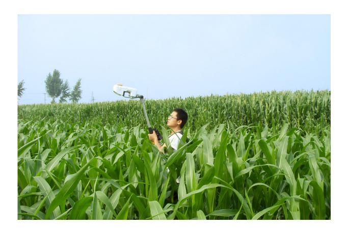
A student uses the GreenSeeker active canopy sensor to collect canopy reflectance data. The collected data will help determine the crop's nitrogen status. Credit: Guohui Feng
