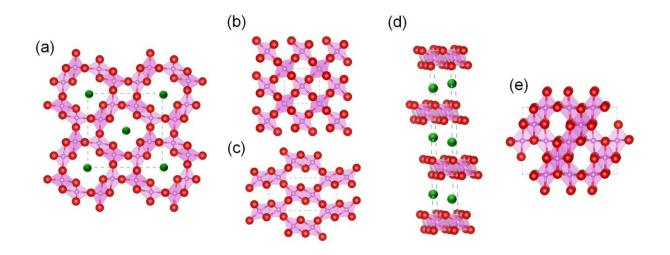
Structures of (a)  $\alpha$ -MnO<sub>2</sub>, (b)  $\beta$ -MnO<sub>2</sub>, (c)  $\gamma$ -MnO<sub>2</sub>, (d)  $\delta$ -MnO<sub>2</sub>, and (e)  $\lambda$ -MnO<sub>2</sub>. Pink, green, and red spheres represent Mn, K, and O atoms, respectively. Of these,  $\beta$ -MnO<sub>2</sub> is the most promising one as a catalyst for oxidation reactions because of the disposition and characteristics of its oxygen atoms. Credit: Keigo Kamata of Tokyo Institute of Technology
