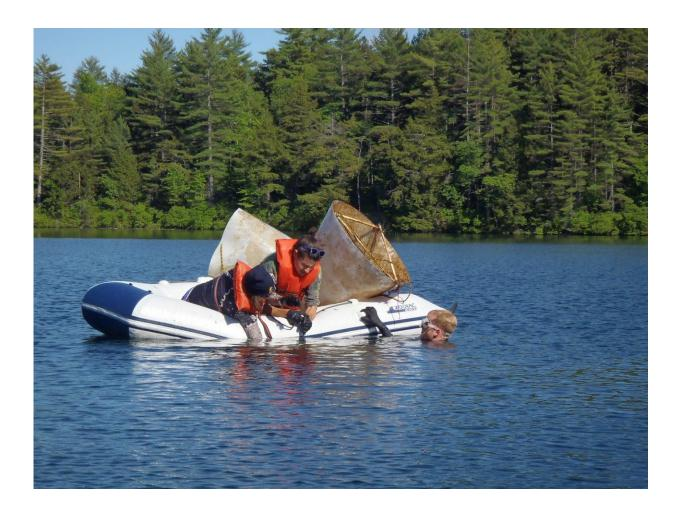
Doctoral students Daniel Miller, in the water, with Helen Habicht and Benjamin Keisling, handle two recaptured sediment traps from an unusually deep lake in central Maine, where they collected 136 sediment samples spanning the 900-year time span to reconstruct the longest and highest-resolution climate record for the Northeastern United States to date. Credit: UMass Amherst
