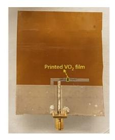
The researchers obtained two thermally and electrically responsive switch configurations on a sapphire surface (left) as well as a tunable antenna operating in two different frequency ranges (right). Credit: Wiley-VCHWiley-VCH
