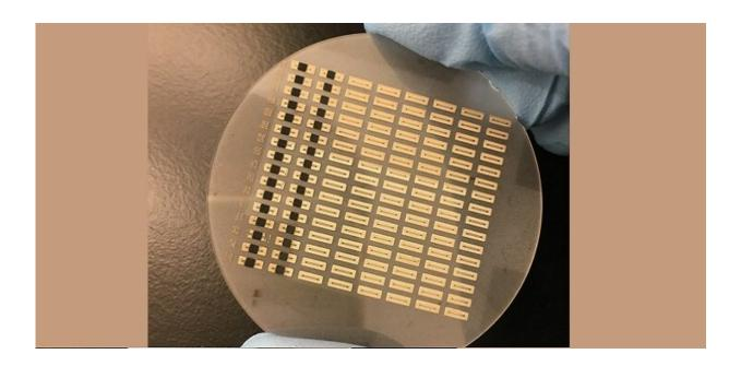
Two thermally and electrically responsive switch configurations on a sapphire surface. Credit: KAUST
