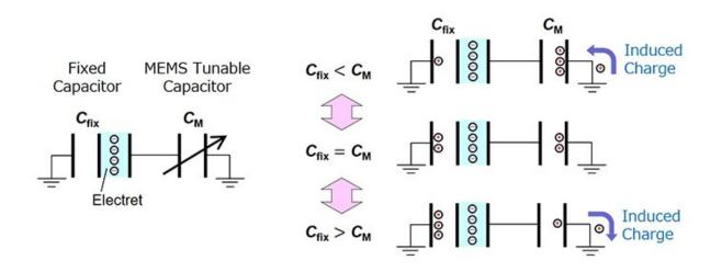
Principle of operation of the proposed energy harvester When the capacity of the tunable capacitor is higher than that of the electret circuit, a movement of charges is induced in one direction. Likewise, when the situation is reversed, a movement of charges is induced in the opposite direction. Credit: Tokyo Institute of Technology
