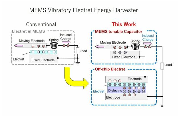
Unlike conventional electret-based MEMS energy harvesters, which contain the entire system in a single chip, the proposed design methodology involves having the electret and the MEMS tunable capacitor in different chips, loosening up design constraints. Credit: Daisuke Yamane
