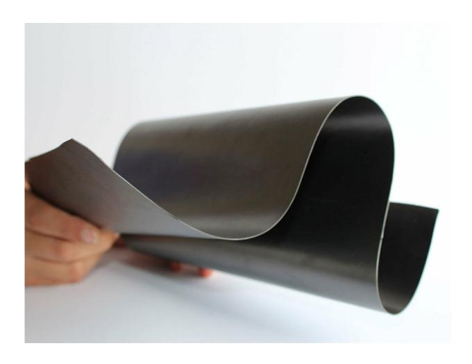
Highly flexible bipolar plate. Credit: Fraunhofer UMSICHT
