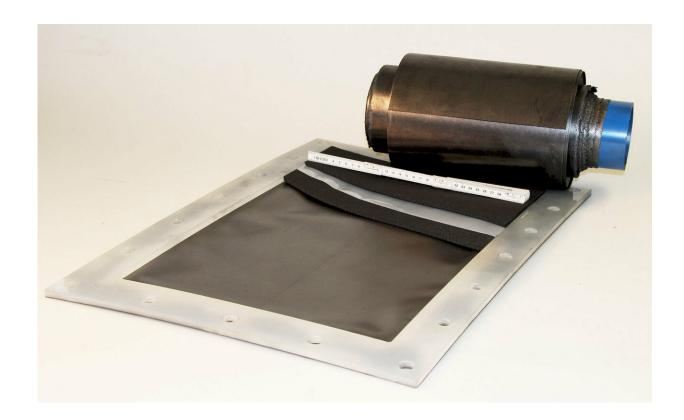
2500 cm<sup>2</sup> redox flow cell and bipolar plate manufactured using roll-to-roll technique. Credit: Fraunhofer UMSICHT
