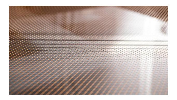
Close-up of the surface of one of the neutrino detector's assemblies, where thousands of wires spaced 3 millimeters apart detect the signals created by neutrinos passing through the detector. Credit: Reidar Hahn
