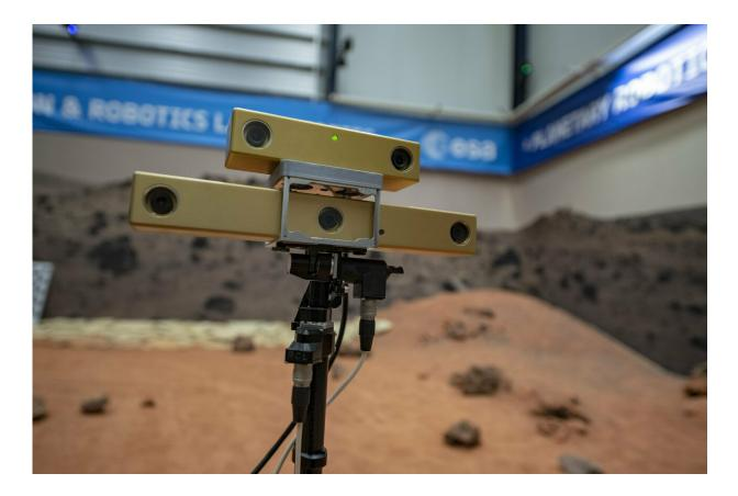
The ExoTeR rover, like the ExoMars rover itself, is equipped with mastmounted stereo navigation cameras for digital elevation mapping. Credit: ESA–G. Porter, CC BY-SA 3.0 IGO
