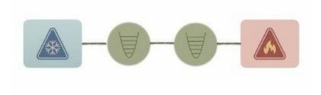
Illustration of a stationary state that is obtained when two quantum harmonic oscillators (in green) are coupled to two heat baths at different temperatures. In this case, a current of heat will flow from the hotter to the colder reservoir, demonstrating irreversible behavior. The experiments described in the study were selected because they conceptually resembled this simplified situation. Credit: Gabriel Teixeira Landi
