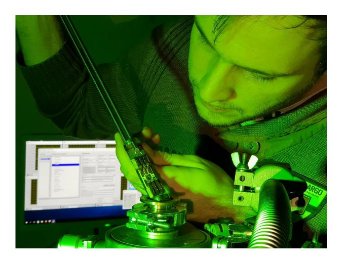
Physicist Martin Hauck fits a silicon carbide transistor into the measuring apparatus: researchers at FAU have discovered a method for finding defects at the interfaces of switches. Credit: FAU/Michael Krieger, Martin Hauck
