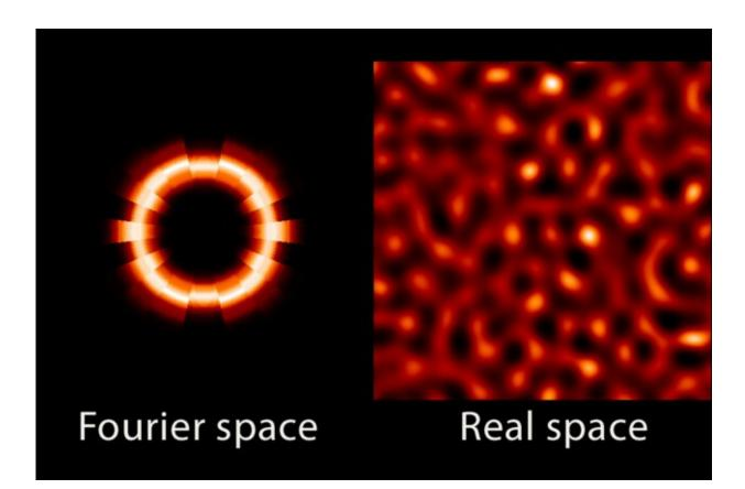
Experiments on ultra-thin copper-oxide ceramic superconductors performed by MIT researchers showed an unexpected disorderly, or "glassy," arrangement of electrons, known as a "Wigner glass." At left, "Fourier space," or momentum space, shows the diffraction data that proved the tendency of the charge ripples to align in any direction, while the image at right displays the random placement of electrons in "real space." Credit: Min Gu Kang
