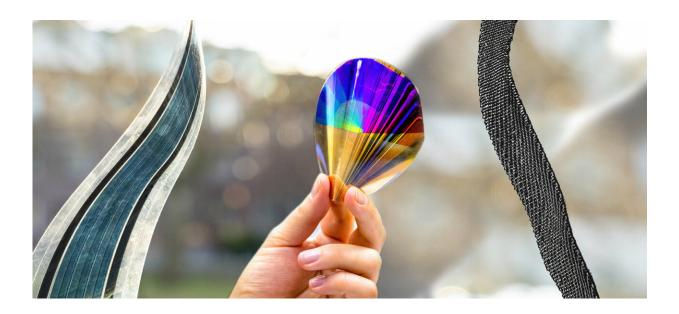
Double doping could improve the light-harvesting efficiency of flexible organic solar cells (left), the switching speed of electronic paper (center) and the power density of piezoelectric textiles (right). (The solar cell was supplied by Epishine AB.) Credit: Johan Bodell/Chalmers University of Technology
