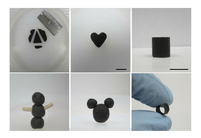
Highly processable and versatile, GO dough can be readily reshaped by cutting, pinching, molding and carving. Credit: Jiaxing Huang/Northwestern University
