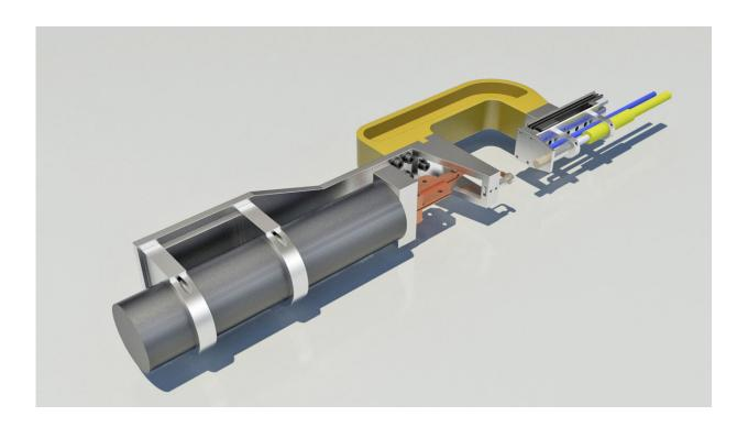
The joining gun bonds metal and plastic in seconds and can be mounted on a robot arm in place of a spot welding gun, for example. Credit: Fraunhofer IWS
