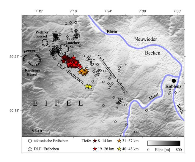
Map of the locations and depths of the deep low-frequency (DLF) earthquakes beneath the Laacher See Volcano ("Lake Laach Volcano") in Germany. Brittle earthquakes are marked as circles, DLF events as stars. Credit: Hensch et al.
